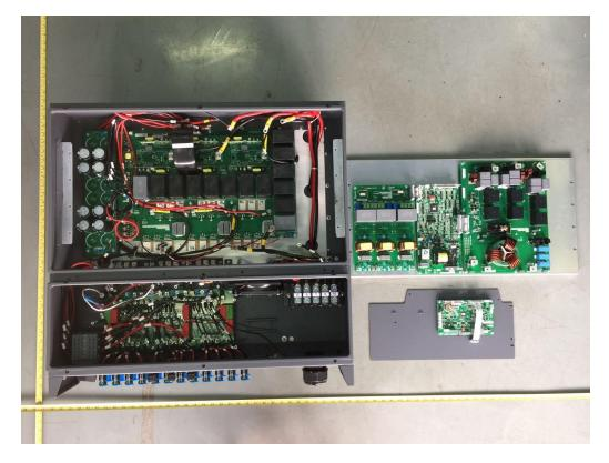
After IP65 test, no deposit of dust and no water are observable inside the enclosure
